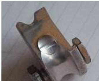
Fig. 9: worn Stop cam
