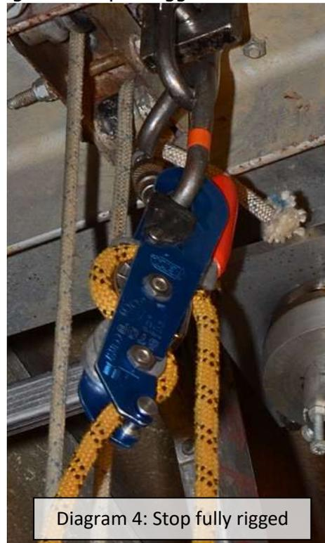
Diagram 4: Stop fully rigged
