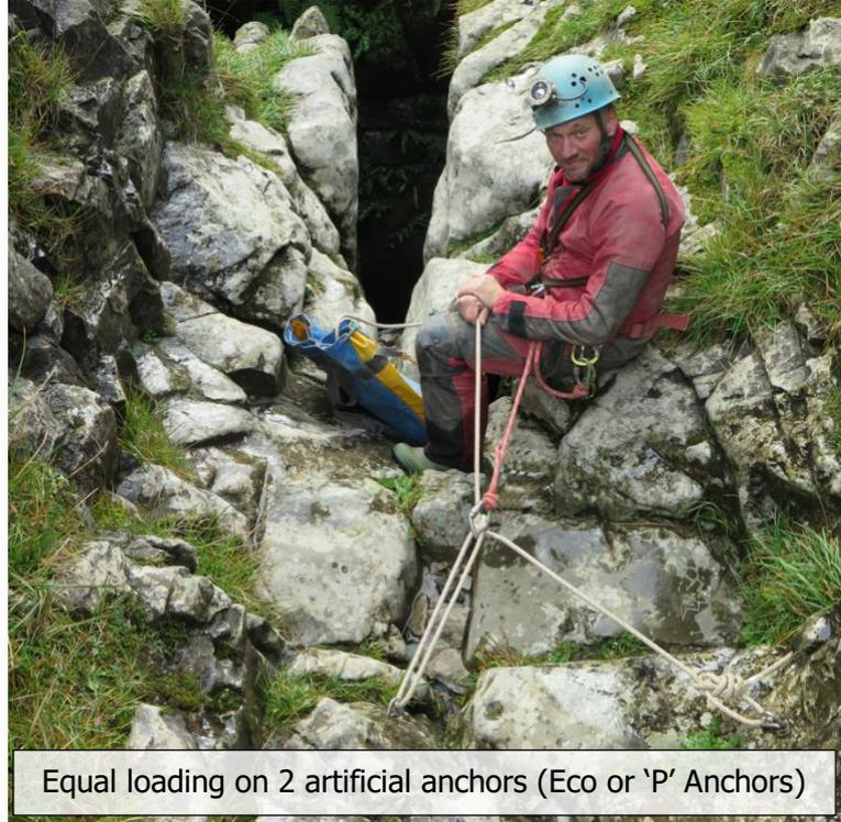
Equal loading on 2 artificial anchors (Eco or 'P' Anchors)
