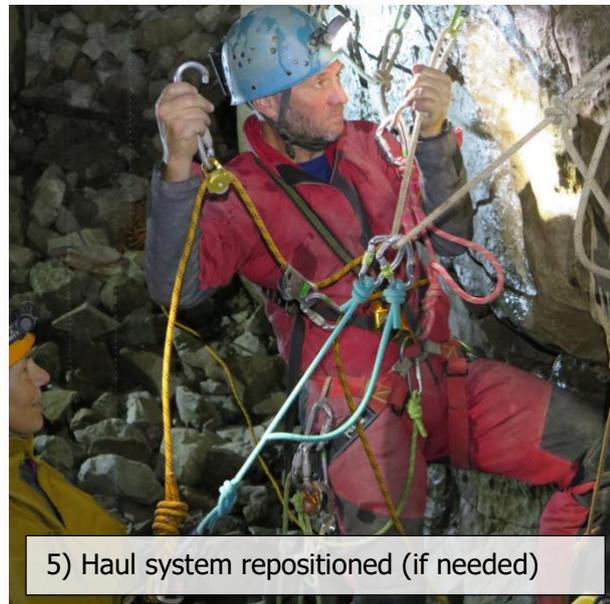
5) Haul system repositioned (if needed)
