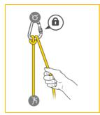
Italian (Munter) Hitch: Useful for short pitches or in an improvised system. Prolonged use, particularly when lowering, can cause the rope to kink significantly and become difficult to handle.
