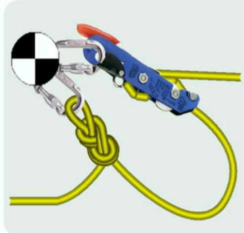
Once tensioned tie the rope directly into the main anchor with 15-20cm of slack. Should the tensioned rope be overloaded the rope should slip slightly through the STOP limiting potentially damaging forces
