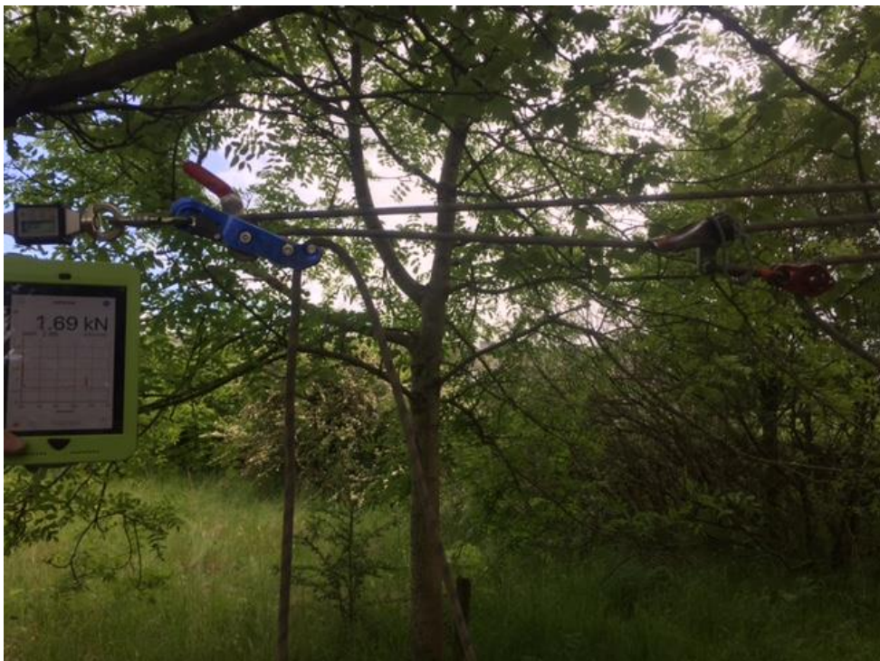
4:1 system two people – after first tensioning (peak reads 2.89kN)
