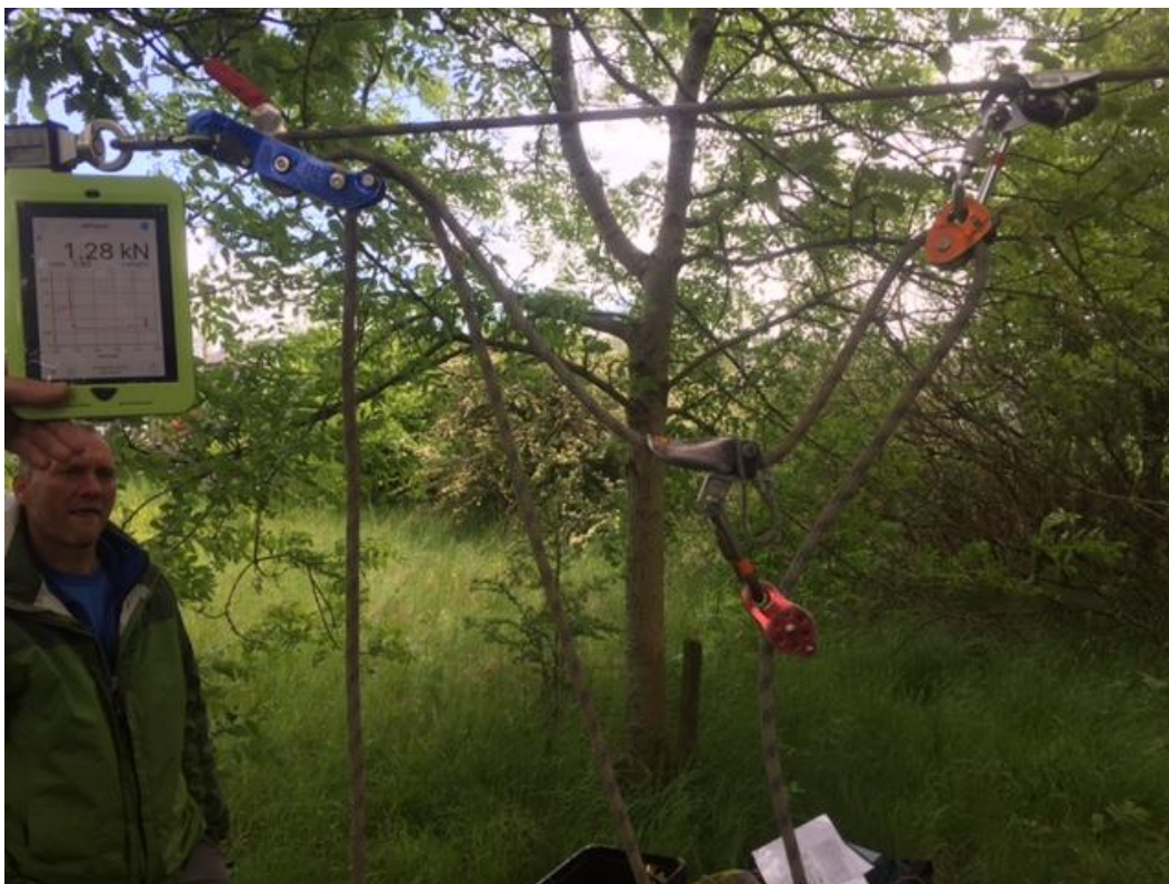
4:1 with central load – reading at anchors (was 1.69kN when first tensioned)
