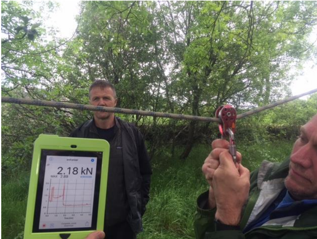
4:1 with central load – reading at anchors (was 1.69kN when first tensioned)
