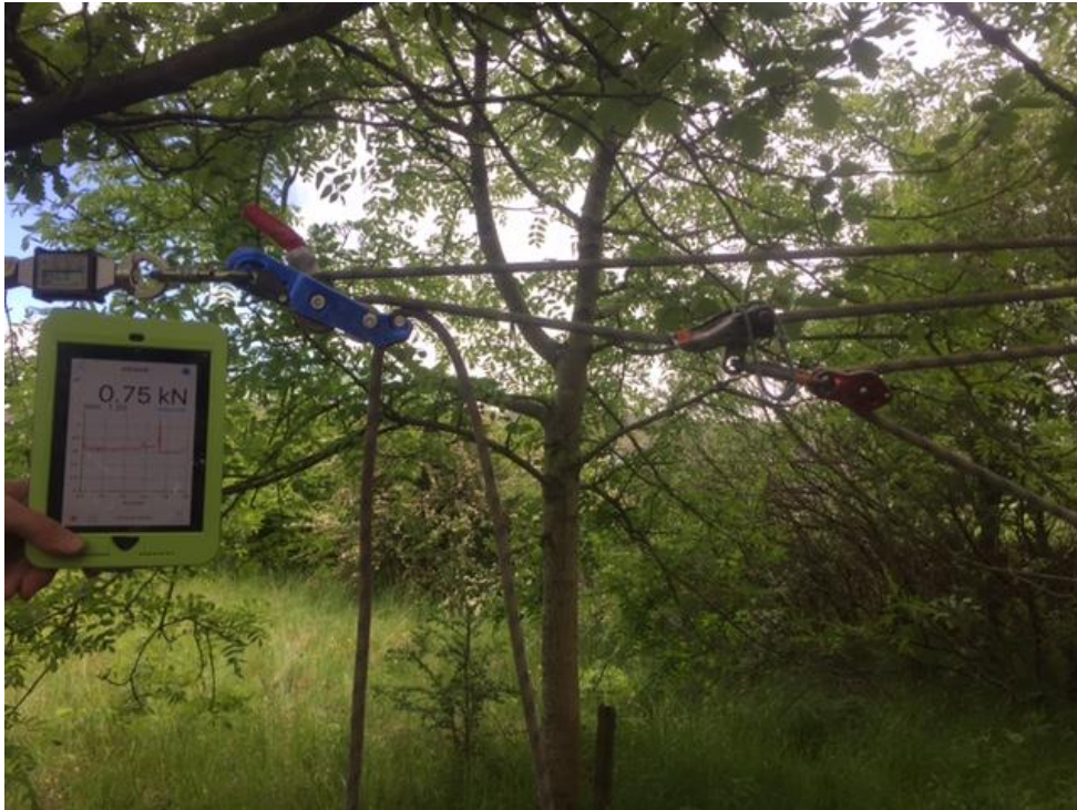
4:1 system – one person settled down (peak reads 1.20kN)
