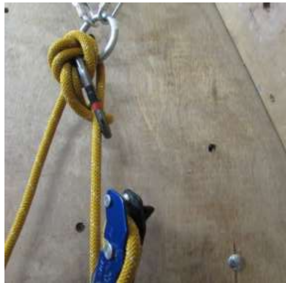
2: Overhand knot and krab through the knot (when using an oversized ring)
