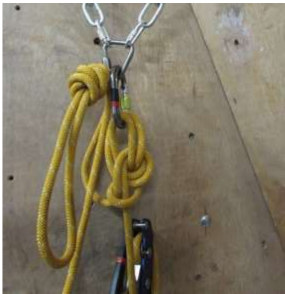
5: Bowline on the bight to tie off rope until last person descends (the bowline unties easily after successive loads)
