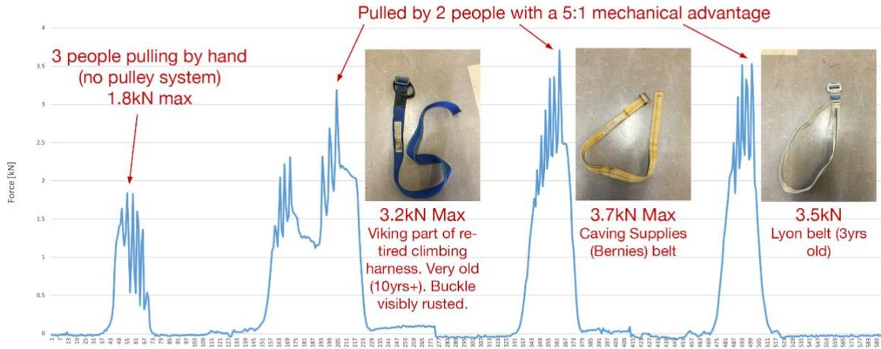
All belts secured around a tree then pulled to at least 3kN. No visible slippage of the belt in the buckle, or damage to the belt following the pull test
