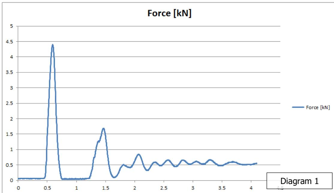
Insulation tape was placed up against the buckle to measure any slippage and the belts inspected afterwards for damage. The belts were subjected to one drop only. The loads were considered to be far in excess of those experienced in any normal use by LCMLA/CIC holders in a working capacity.
