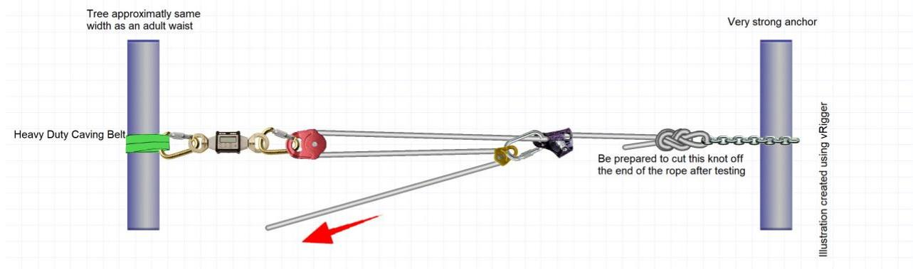
We also used a Petzl Rollclip to redirect the angle of pull to make it easier to stand on the tarmac of the road alongside the trees.
