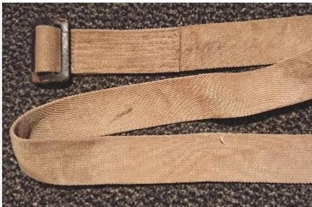
Age questionable, however no significant fraying. Buckle showing some corrosion. May be suitable for use but requires monitoring
