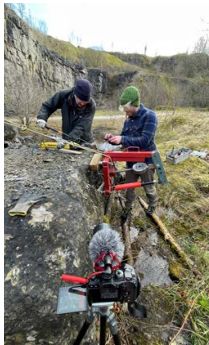
The BCA heavy duty anchor puller in action at Horseshoe Quarry Photo: Pete Knight
