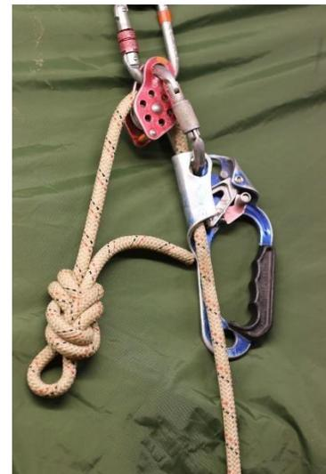
Before and after of a pulley and ascender combination for life lining drop test © G Thomas
