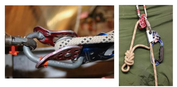
Before and after of a pulley and ascender combination for life lining drop test © G Thomas
