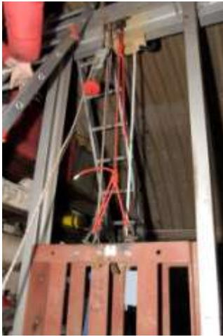
**Figure 1 Rig Set up showing Double Bowline on Bight**
